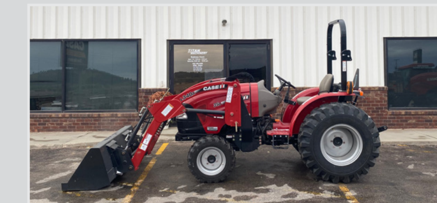
2981392 2022 Case IH Farmall 35A, 5 Hrs, Hydrostatic Trans, 43x16.00-R4 Rears, 25x8.5-14 Fronts, 1 Remote, Loader, 540 PTO, Call
