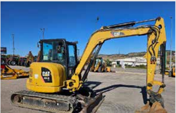
3309671 2012 Caterpillar 305.5E, 6235 Hrs, 10,000lb Op Weight, Cab/Air, Aux Hyd, Mech Coupler, Blade, $39,900
