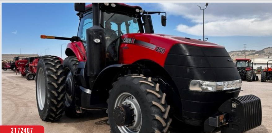
2020 Case 250 3965 Hrs 19-Spd Pwr Shift, 480/80R46 Rear Duals, 420/90R30 Fronts, Guidance Ready, 4 Remotes, 1000 PTO, Std Pump 3172407 183380
